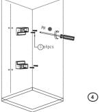
4. After anchor screws have been installed, install Positioning and Support Wall Mounting holders #6 using supplied screws #8.
