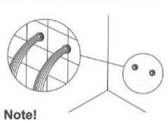
Before assembly, flush the water supply pipes thoroughly to remove debris(allow the water to run with the main stopcock open for about 3 mins), otherwise dirt particles might affect the function of the shower panel!
